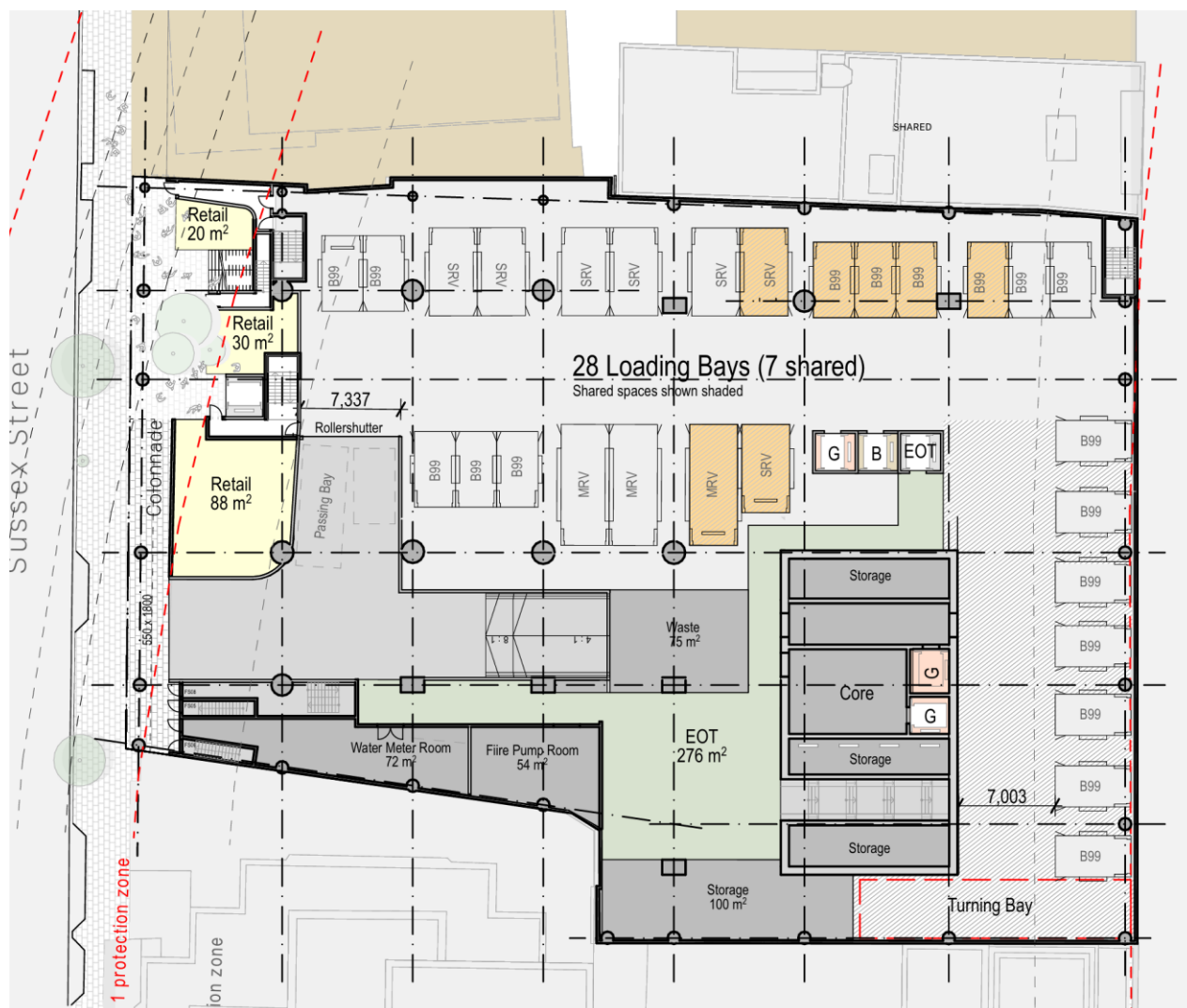
Figure 1: Reference Loading Dock Arrangement
